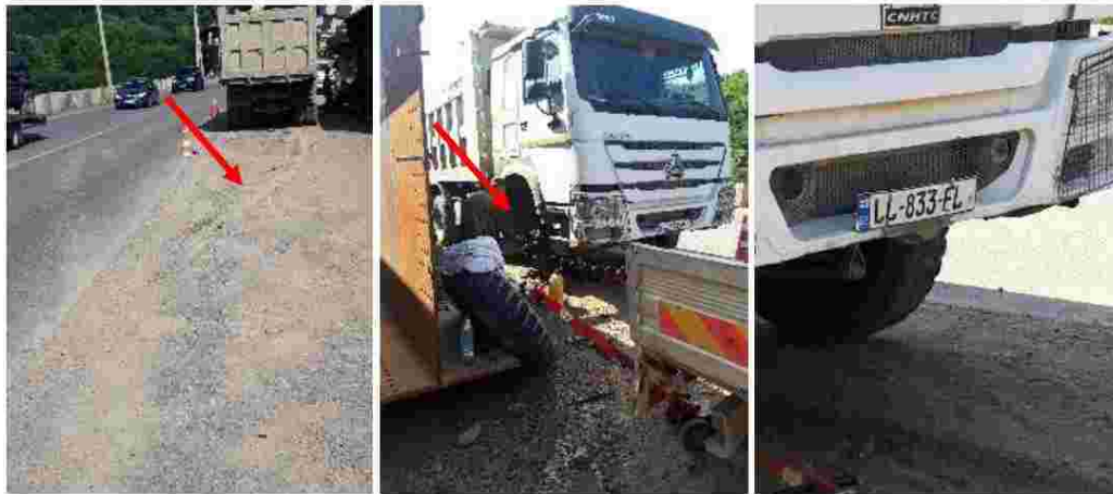
Picture 12: Negative Observation – Driving safety (Main road (E60)) – Additional attention to the Company trucks must be paid from the Contractor's side, because the use of damaged and not properly repaired trucks may cause the traffic related accident and possible personal injury of the drivers and pedestrians as well. One of the examples has been given in the pictures attached below. The tire became loose on the truck while it was moving. Nobody got injured and it didn't cause the traffic accident as well. The Contractor has to pay additional attention to this issue in order to avoid the possible incident and injury of the working personnel. Non-compliance isn't solved.
